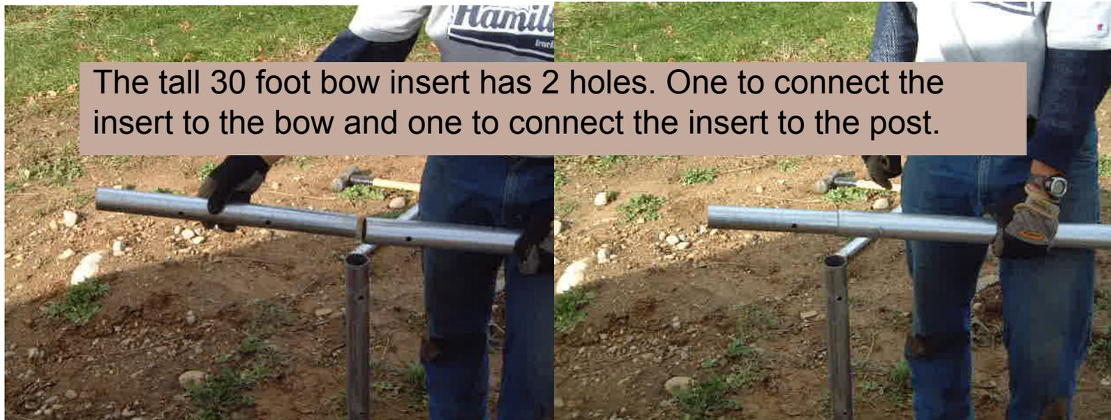
The tall 30 foot bow insert has 2 holes. One to connect the insert to the bow and one to connect the insert to the post.
